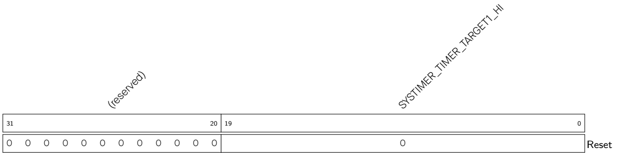
Register 11.18. SYSTIMER_TARGET1_HI_REG (0x0024)
