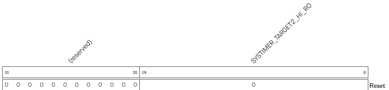
Register 11.35. SYSTIMER_REAL_TARGET2_HI_REG (0x0088)
